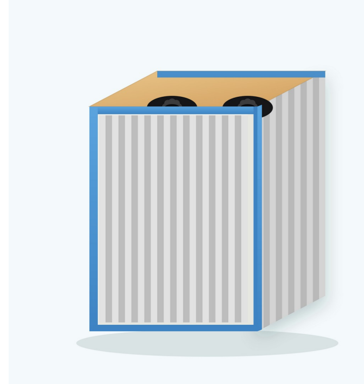
MERV-13 filter walls, fans on top
